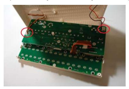
**Step 4:** Choose a location to mount the VolcaMod MIDI OUT modificator on your Volce-series device. We suggest above the original "MIDI IN" socket, but of course it can be mounted in various other locations throughout the device where clearance is suitably available.
