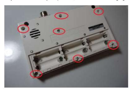
**Step 2:** Carefully open the bottom cover from the top cover as wires will be attached.
