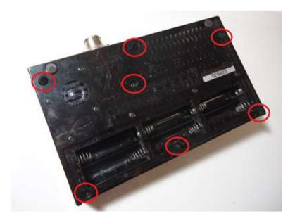
**Step 2:** Carefully open the bottom cover from the top cover as wires will be attached.
