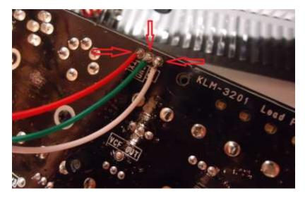
**Step 10:** Carefully tuck the loose wires back into an appropriate position and close the bottom cover and the top cover.
