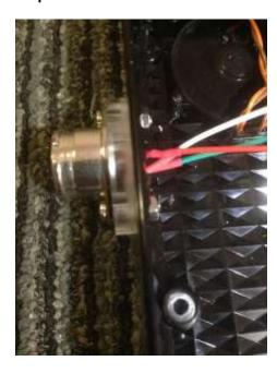
Step 9: With a soldering iron, reconnect the wires for battery and speaker.
