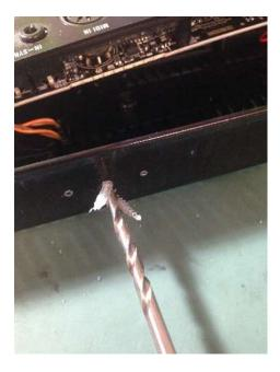
**Step 7:** Use a 9mm drill bit and drill the center hole. (**Carefully** do this, as forcing the drill bit is likely to crack the case)
