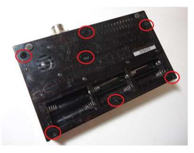
Step 2: Carefully open the bottom cover from the top cover as wires will be attached.
