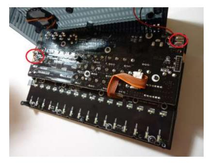
**Step 4:** Choose a location to mount the VolcaMod MIDI OUT modificator on your Volce-series device. We suggest above the original "MIDI IN" socket, but of course it can be mounted in various other locations throughout the device where clearance is suitably available.
