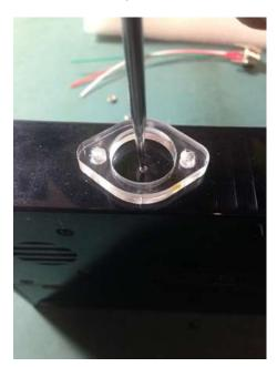
**Step 6:** Drill a 3.5mm drill bit and drill the holes. (**Carefully** do this, as forcing the drill bit is likely to crack the case)
